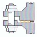
Spiral Wound Gasket with sealing element and Inner ring only. Mainly used for male and female flanges and recess flanges. The inner ring is necessary as a compression stop.
